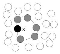
Figure 2.6: Home node and perimeter in Data-Centric Storage
