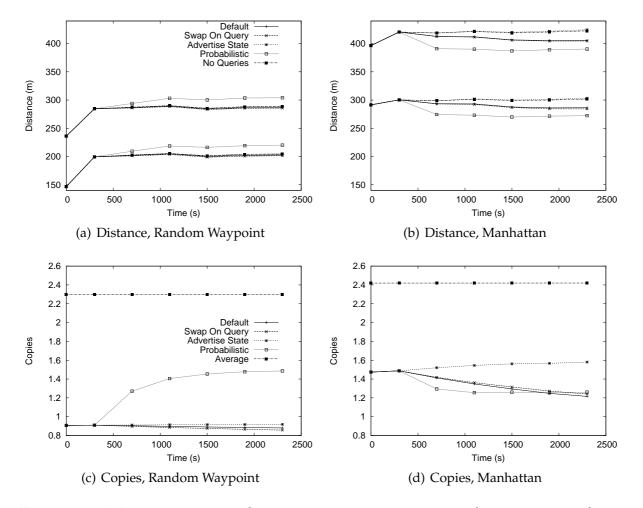
Figure 4.36: Mitigation tests with 250m transmission range, 5m/s average speed, 700 items and DbC=2
