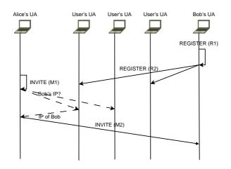
Figure 5.5: Simplified logical message flow in SIPCache
