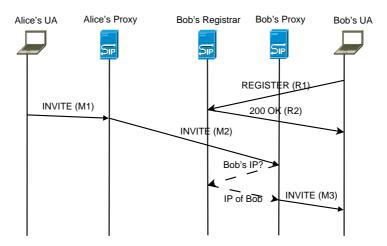
Figure 5.1: Simplified logical message flow in SIP
