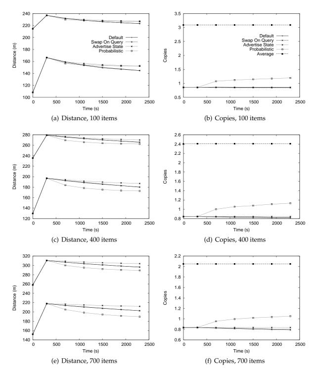
Figure 4.28: Convergence tests when *DbC*=2 and transmission range=300m
