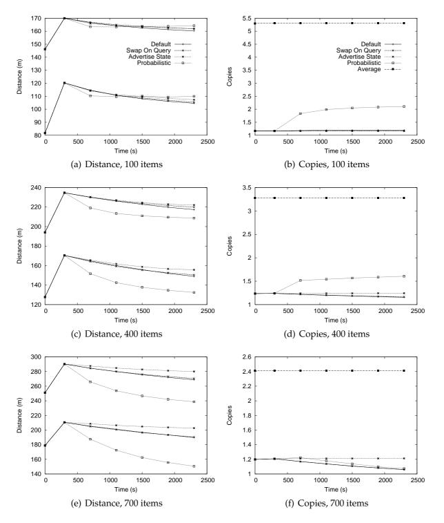
Figure 4.26: Convergence tests when *DbC*=2 and transmission range=200m
