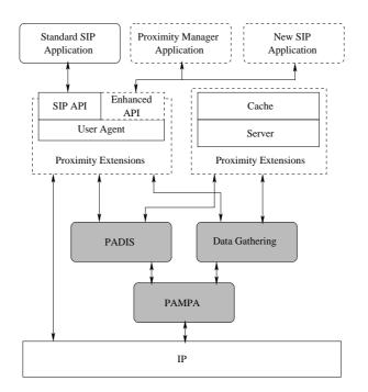
Figure 5.4: Software architecture for SIPCache
