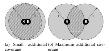
Figure 2.18: Overlap of the coverage of the transmission range between two nodes
