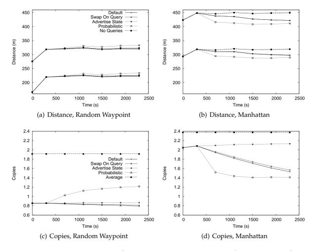
Figure 4.34: Mitigation tests with 200m transmission range, 5m/s average speed, 700 items and DbC=4
