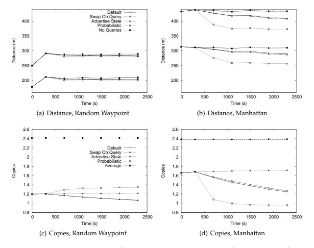
Figure 4.33: Mitigation tests with 200m transmission range, 2m/s average speed, 700 items and DbC=2
