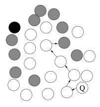
Figure 2.3: Intersection of trails and queries in rumour routing
