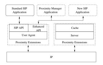
Figure 5.2: Software architecture for decentralised SIP
