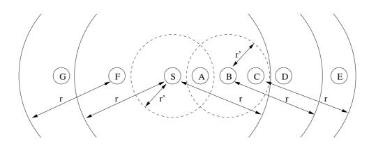
Figure 3.1: Deployment and transmission range of some nodes
