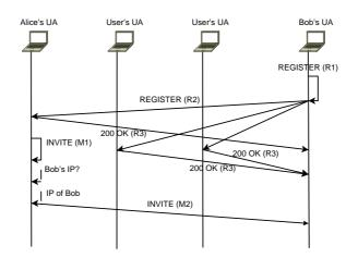
Figure 5.3: Simplified logical message flow in dSIP
