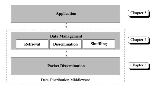
Figure 1.1: Architecture of data distribution middleware frameworks
