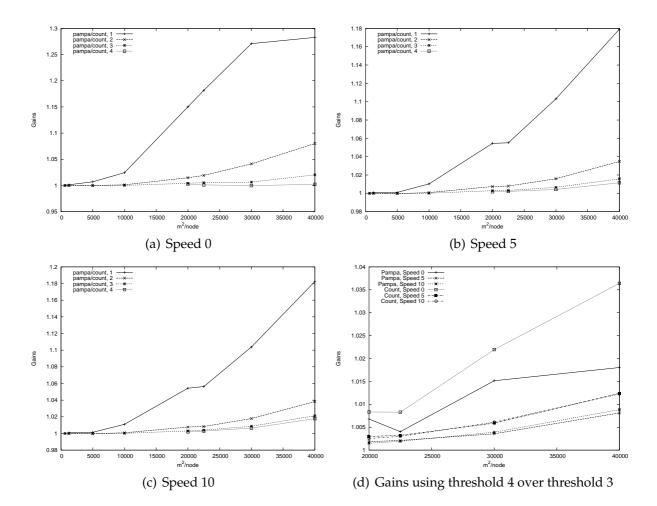
Figure 3.6: Comparison of the delivery ratio of Pampa with the "counter-based scheme"
