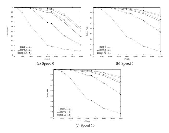
Figure 3.5: Delivery Ratio of Distance Based algorithms
