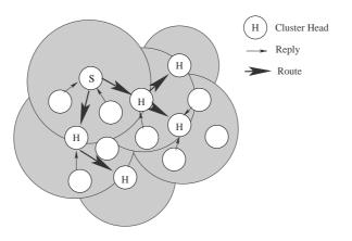
Figure 5.8: Propagation of gathering messages and replies
