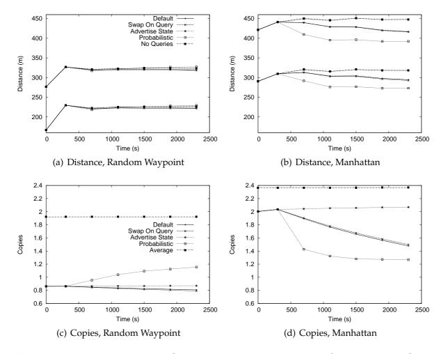
Figure 4.30: Mitigation tests with 200m transmission range, 2m/s average speed, 700 items and DbC=4
