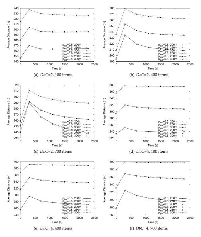
Figure 4.25: Average distance of the nodes to the closest replica for two configurations of the Probabilistic algorithm
